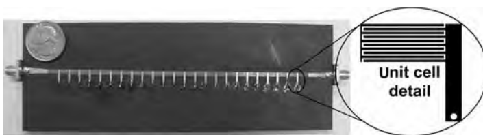
FIGURE 3.6 Microstrip CRLH transmission line implemented by means of shunt-connected grounded stubs and interdigital capacitors. (Source: Photo courtesy of C. Caloz.)
